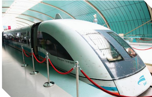
Maglev (magnetic levitation) trains can travel more than 400 kilometres per hour. The strong magnets between the train and the tracks repel each other, causing the train to 'float' above the tracks. Other magnets allow the trains to move at great speeds. Why is the distance between the 'floating' train and the tracks important? What could happen if it is too short or too long?
