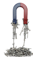
Magnetic force can act over a distance to attract the iron nails.
