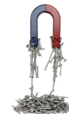
Magnetic force can act over a distance to attract the iron nails.
